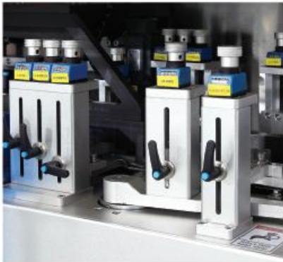
▲ 数显调节机构 Digital display regulating mechanism
