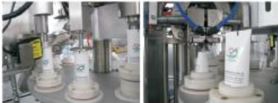
软管计数检测装置 Tube count and check device
