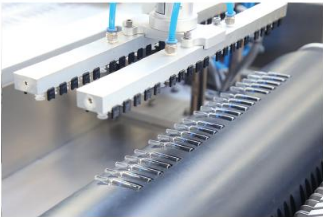
▲ 伺服机械手装置 Servo Mechanical hand
