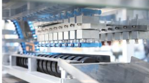
▲ 机械手自动摆料 Mechanical hand automatic feeding
