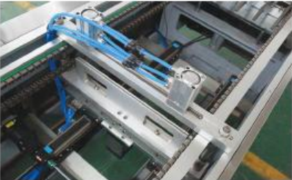
▲ 伺服电机齿形横向切刀装置 Cross cut for bevel shape packing by servo motor
