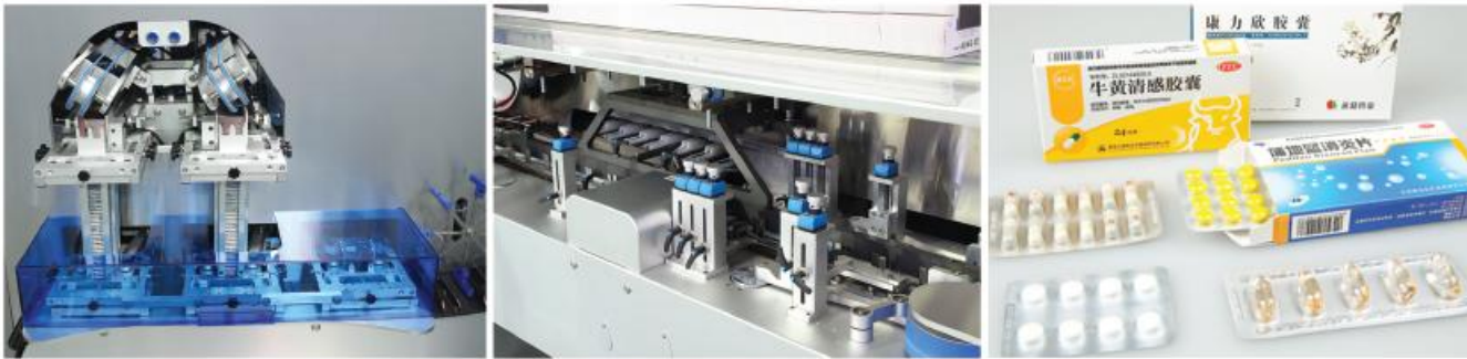
▲ 装盒机加料机构 Feeding mechanism
