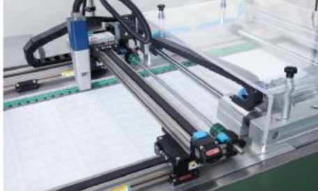
▲ X、Y轴喷码装置 Ink jet printing with X,Y direction
