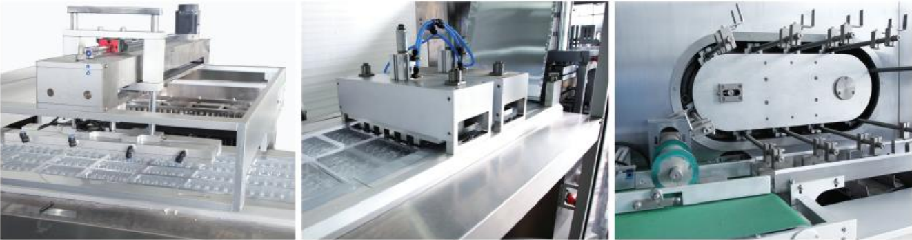
▲ 伺服机械手装置 Servo Mechanical hand
