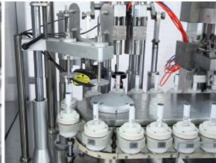
双计数、对标装置 Double count, double eye mark device
