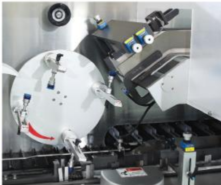
▲ 高速吸盒机构 High speed box sucking device
