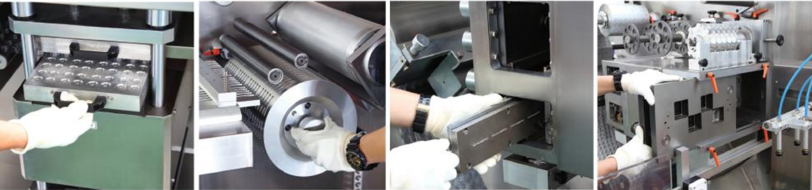
▲ 无工具更换成型模具 Change forming mould without tool
