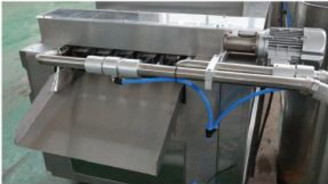
▲ 收废边装置 Waster edge collecting device
